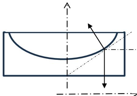
$$N_x = -mg \cos \varphi \sin \varphi \cong -mg \tan \varphi = -mg2ax. \quad (2.1)$$
